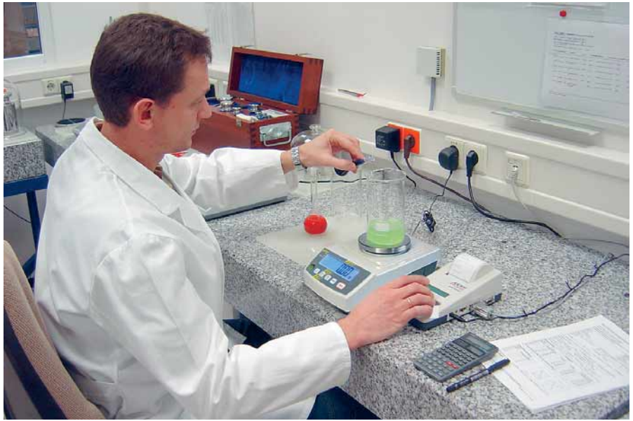
Weighing plate A ring-shaped draft shield standard, Ø 90 mm, height 53 mm
